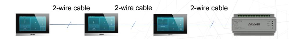
Support the daisy chain wiring mode and make full use of the wiring of original analog intercom
