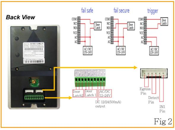
2.1 According your door lock type, see wiring diagrams below.
