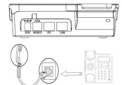
PC port to PC, LAN port access outside the network, EXT Socket Extension units, SOR (PSTN) port access PSTN, Upper right to power, the right of access RJ11 headset, the lower right of access a handset.
