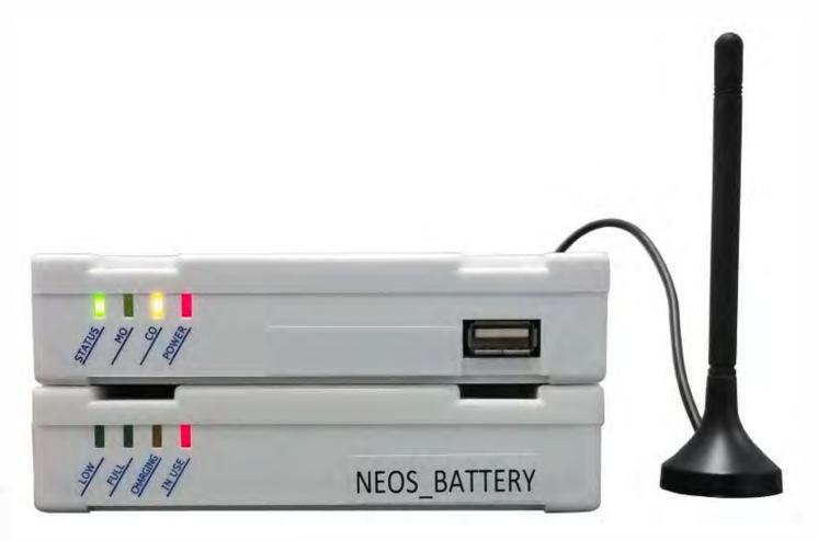
NEOSLIFT Voice gateways provide a replacement for analogue telephone lines connected to elevator phones.
